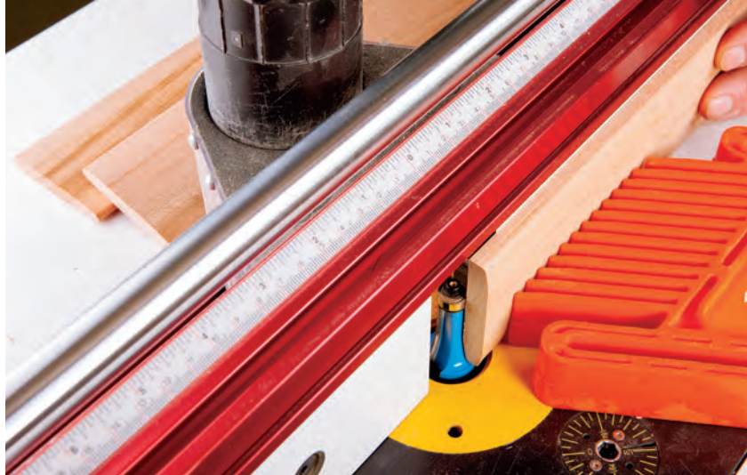
An optional louver-shaping router bit can mill louver blanks from any wood species at the router table. Our author was pleased with its performance. Premilled basswood louver blanks and rail and stile stock are also available if you'd prefer not to build shutters completely from scratch.
