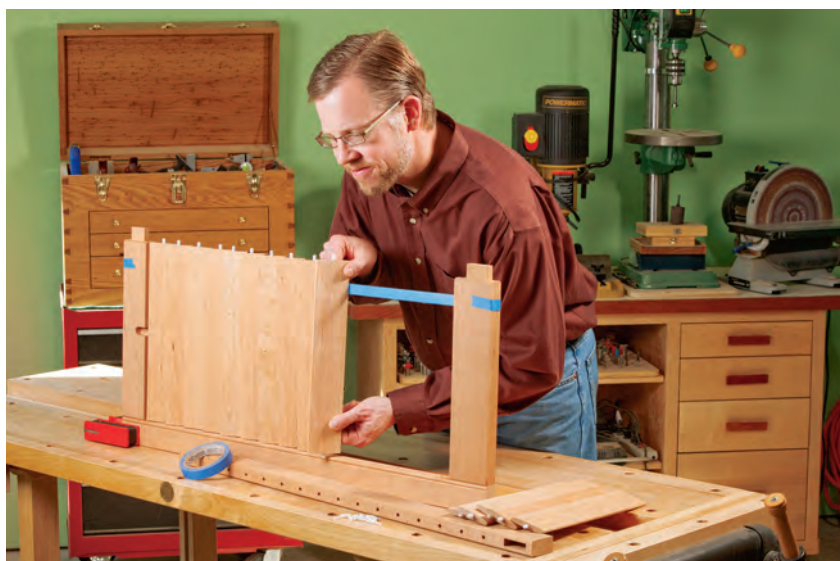
Movable louvers, as shown here, swivel on single pairs of pins inside the shutter frame. A wood control arm and metal clips (not shown) move them all in unison. Fixed-louver options either use two pins per end or are housed in routed mortises instead. The author found that a long strip of tape was convenient for holding the louvers in position during dry-fit and assembly.
