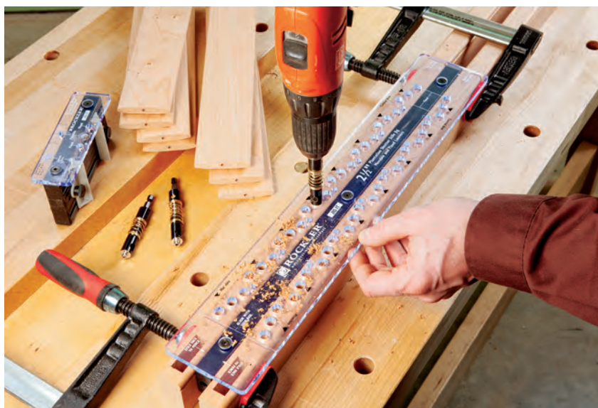
Louvers mount on the shutter stiles with plastic pins. Two sturdy jigs that come with the kit enable accurate hole drilling in the stiles and louvers with three sizes of self-centering bits.
