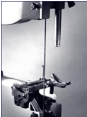
Delta band saw with table and original guides removed
