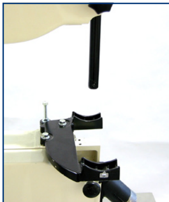
Jet band saw with table and original guides removed
