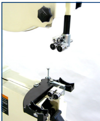
Jet band saw with new guides attached
