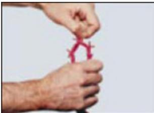
Hold belt upside down. Bend back as far as possible; hold with one hand. Twist one tab 90° parallel with slot.
