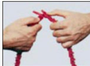
Rotate belt end with tab 90°.
