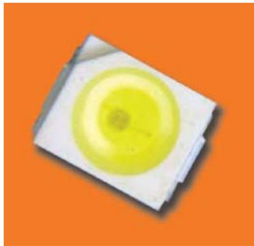
The White source color devices are made with Gallium Arsenide Phosphide on Gallium Phosphide White Light Emitting Diode.
