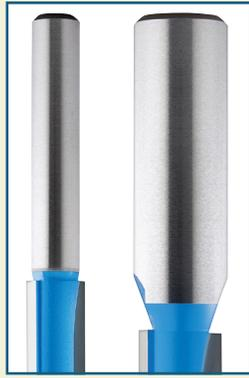
**Third, most router bits have solid-carbide or carbide-tipped cutting edges.** Most of the profile bits will have carbide cutters, which are harder than steel and will hold an edge longer – 10 to 25 times longer – but also are more brittle. So while carbide-tipped bits are preferable, you must handle and store them carefully to avoid chipping the cutters.
