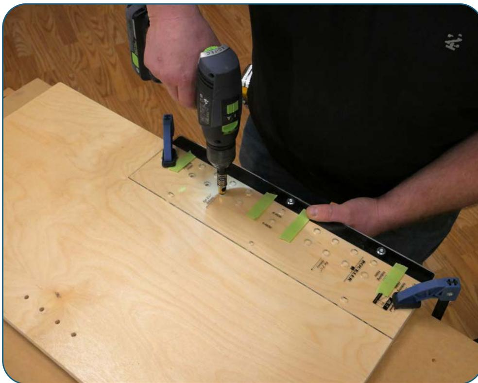
Use a shelf pin drilling jig (31571 or 32991) to drill the shelf pin holes.
