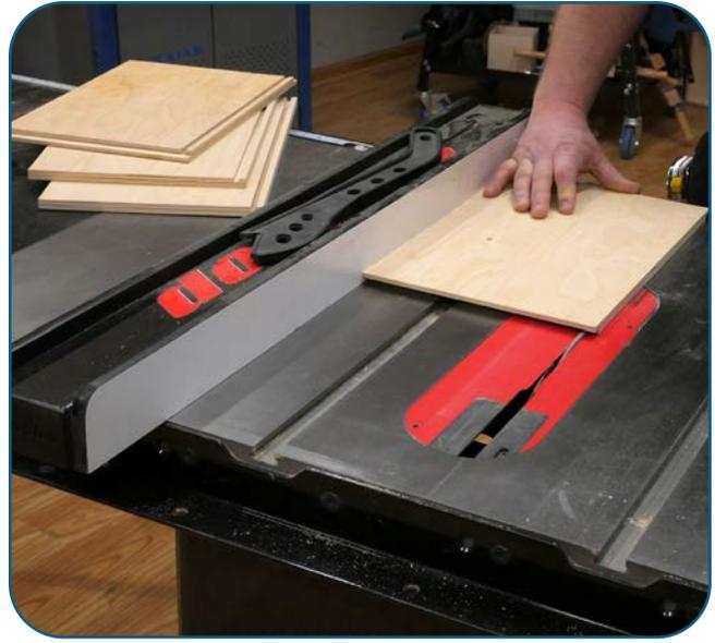
Cut a 1/4"-wide x 1/4"-deep groove in the inside faces of the drawer front, back, and sides. This groove will capture the bottom panel.
