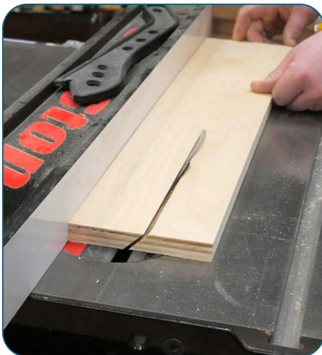
Tilt the table saw to 45 degrees. Rip the French cleat rails.
