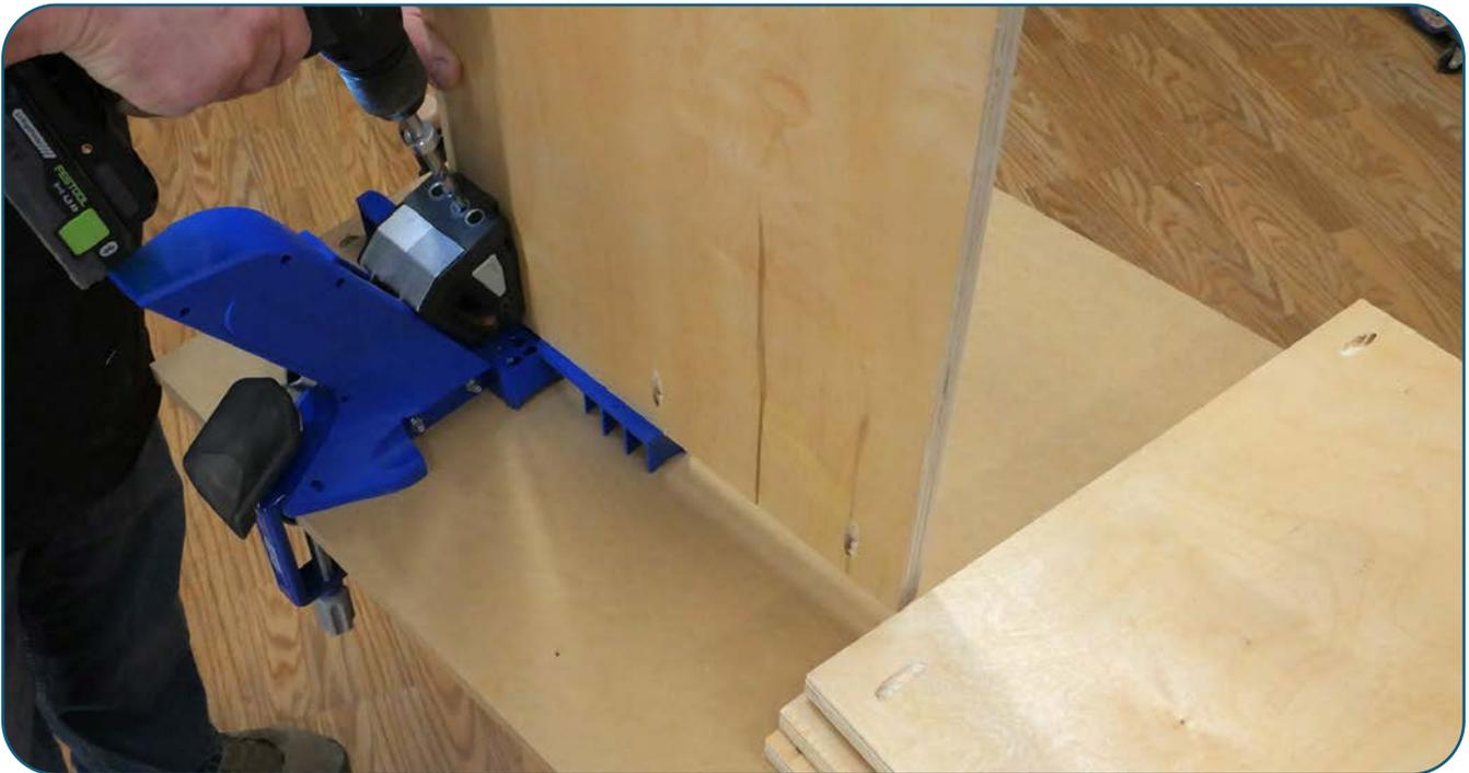
Drill pocket holes along the side edges of the top and bottom panels.
