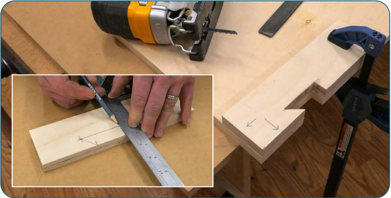
Make a French cleat bracket template. Lay out the french cleat bracket on a piece of scrap wood. See layout drawing, p.2. Cut out the French cleat bracket with a jigsaw. Use the template to layout the French cleat brackets on each side panel.
