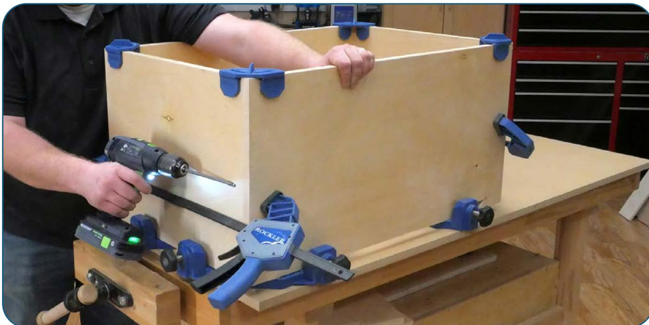
Clamp the top, bottom and sides of the case. Assemble with 1-1/4" pocket screws into the pocket holes.
