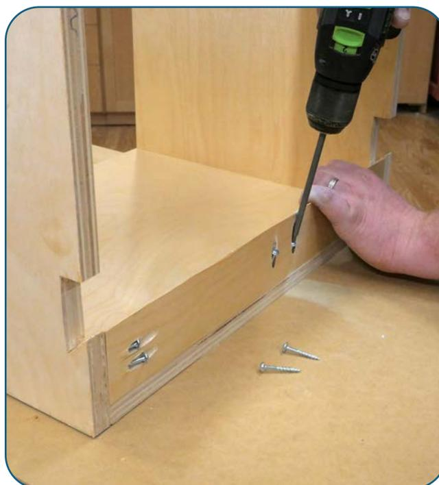
Cut the French cleat rails to length. Drill pocket holes in the ends and attach the rail to the cabinet case.
