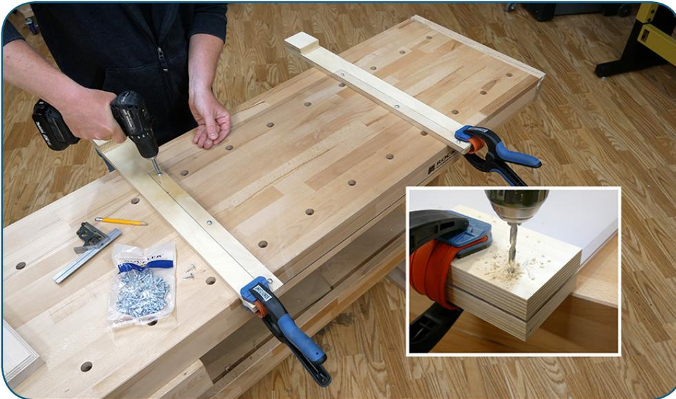
Drill  $\frac{3}{16}$ "-dia. pilot holes through the acrylic sheet. Evenly space three holes  $\frac{3}{4}$ " in from the side edge of the acrylic. Clamp the acrylic between two pieces of scrap wood to prevent chipping or cracking when drilling the holes (inset). Position the acrylic to overlap the inside edge of the Posts by  $1\frac{1}{4}$ ". Attach the acrylic sheet to the posts with #8 x  $\frac{3}{4}$ " truss head, pan head or washer head screws.
