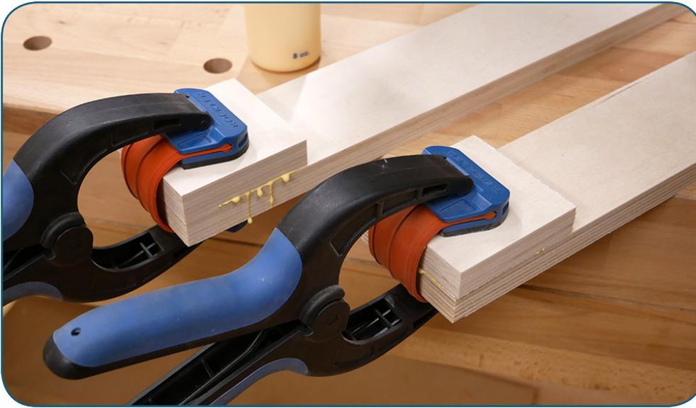
Cut your Posts and Support Blocks to length and width. Glue and clamp a Support Block to the end of each Post. After the glue has cured, sand all surfaces and apply the topcoat finish of your choice.
