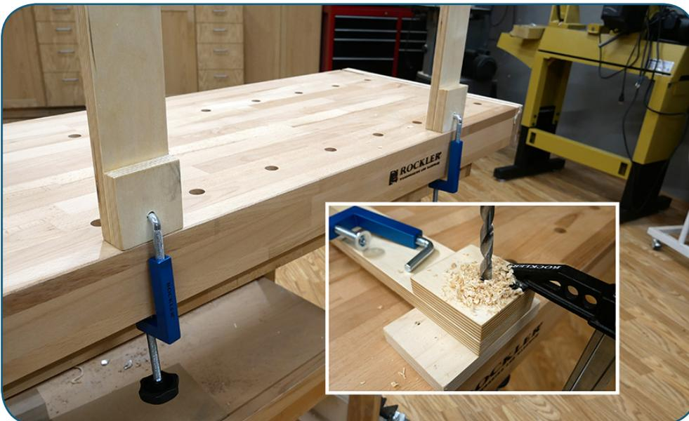
The final step is to drill a  $\frac{3}{8}$ "-dia. hole located 1" up from the end of each Post (inset). Install a Rockler Universal Fence Clamp in each hole and secure the guard to a countertop or table. This guard will clamp to countertops up to 5" thick.
