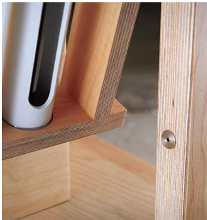
The metal disk shown at left aligns with a rare-earth magnet epoxied into the bottom end of the tool holder (hidden from view). This keeps the tool holder upright when you roll the cart around the shop. The author uses the jig at right to rout the little windows in the PVC tubes.
