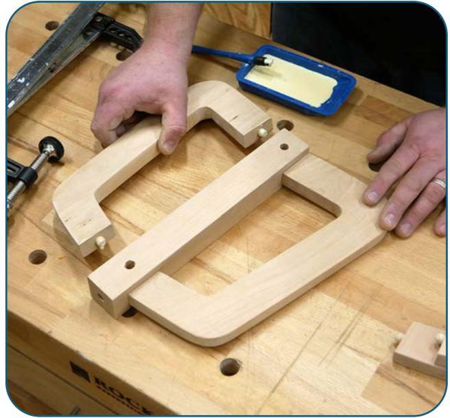
Connect the legs to the center post with glue and dowels.
