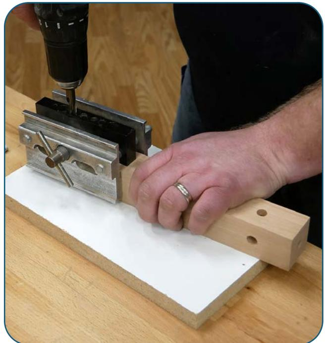
Use a Self-Centering Doweling Jig to drill the dowel holes in the center post.
