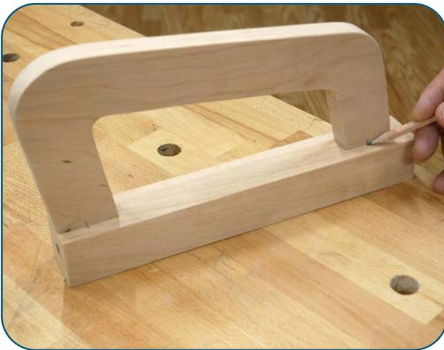
Position one of the legs on the center post and transfer the dowel locations on the center post.
