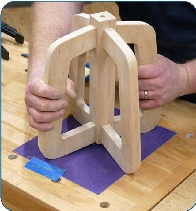
The legs are likely to not be perfectly level with each other and the lamp may rock slightly. Tape a piece of sandpaper to a flat surface and sand to four legs until they are level.
