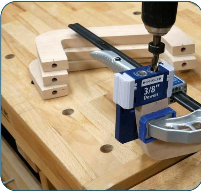
Use the Rockler Doweling Jig to drill the 3/8" dowel holes in the legs.
