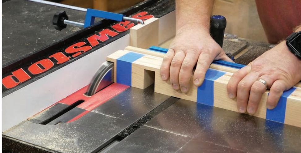
*Group the eight filler slats and back slat into a bundle with painter's tape, carefully aligning the part ends. With your dado blade raised to 1 3/4", cut 1"-wide dados for the two middle supports and a 3/4"-wide notch into each end, leaving 1/4" tongues.*
