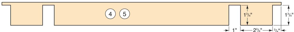
We still need to cut a 1/4"-deep, 3/4"-wide notch into the top back corner of this bundle to finish the cross-lap joint with the back slat, so install your
