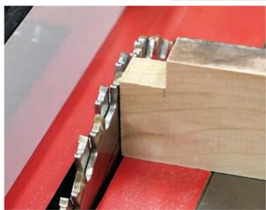
*Use the front slat as a reference for setting blade height (inset) before milling a 1 1/2"-deep notch into one end of the middle/end support bundle. The other end receives a 1/4" x 3/4" notch.*
