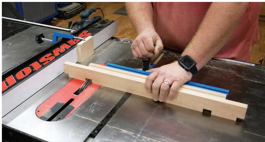
**Mill 3/4"-wide, 1/2"-deep notches into the ends of the front slat, using a step-off block clamped to the rip fence for both indexing and safety. Then reset the fence to cut 1"-wide dados for the shelf's two middle supports. Position these 3 1/2" in from the part ends before cutting them.**
