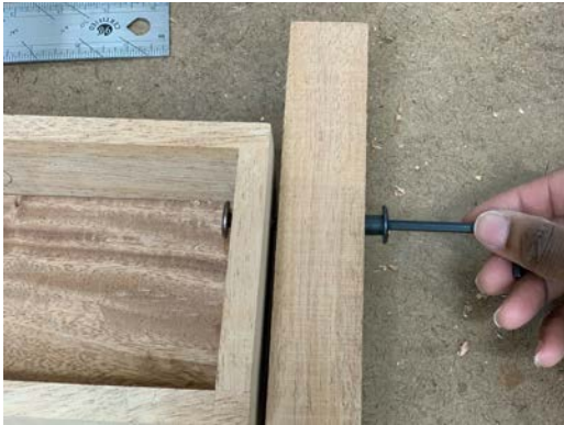
Join the base and pole together with 1 ¼" screw
