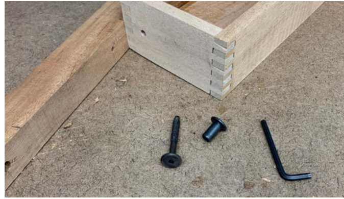
Drill ¼" holes on both sides of each box
