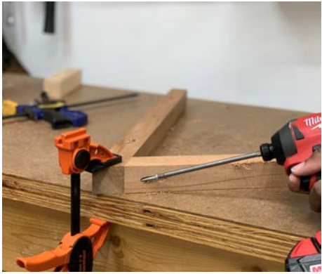
Join the base and pole together with 1 ¼" screw
