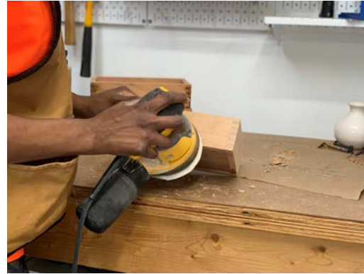
Sand all surfaces with 150 and 220 grit sandpaper
