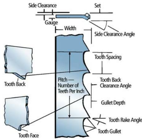
**Flex Back** – Saw blade with hardened teeth but a relatively soft back.
