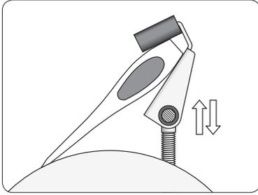
Place the axe into the jig. Set the edge angle by adjusting the Universal Support. Either at the original angle using the Marker Method or at a new angle using the AngleMaster WM-200.
