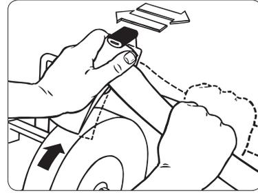
Follow the shape of the edge (straight or curved) during grinding by raising or lowering the handle. Let the jig slide sideways on the Universal Support so that the stone wears evenly.
