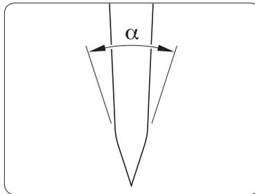
A felling axe should have an edge angle ( $\alpha$ ) of 30–40°. Round off the heels and the axe cuts more easily.
