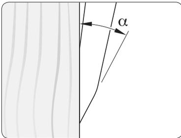
Put a longer bevel on the wood-side on a carpenter axe.
