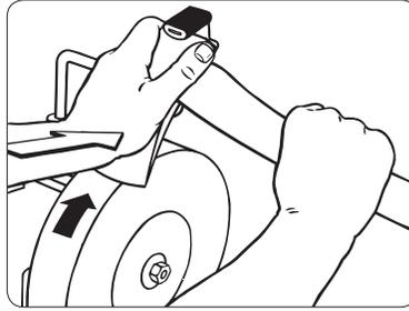
Press with your palm on the axe, close to the stone. The axe will automatically be pressed up against the stop in the jig and the grinding is most efficient.
