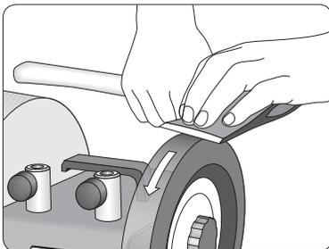
Honing and polishing the bevels on the leather honing wheel makes the edge cut more easily and the sharpness will stay longer. Always hone away from the edge.
