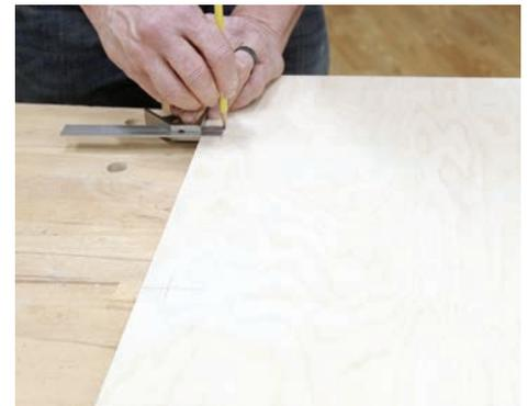
3) Place a cross mark on each hinge centerline on the lid. This will locate the cup hinges on the inside of the cabinet lid.
