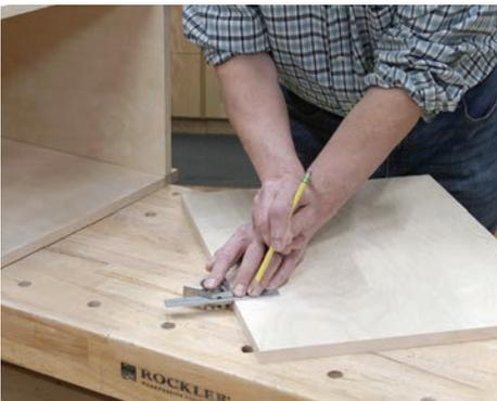
1) This system mounts onto a 35 mm hinge set from Sugatsune. Determine the spacing of the hinges and mark their locations by drawing a centerline for each hinge component.
