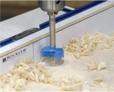
7) Chuck a 35 mm Forstner bit into the drill press. Set the depth to 11 mm into the 3/4" lid. Bore the holes at the marked locations.
