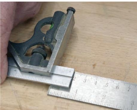
4) Reset the depth of the combo square to 19 millimeters.
