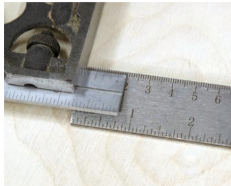
2) Set the depth of the combo square to 20.5 millimeters. Here the measurement is transferred to a combo square.
