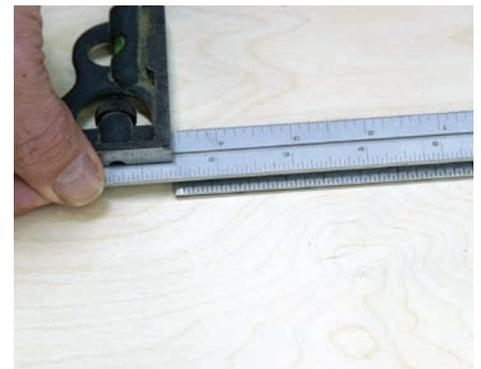
6) Reset the combo square to 118 mm. Choose which side to mount the lid stay. Extend that hinge centerline and mark a cross line where the lid stay will attach to the lid.
