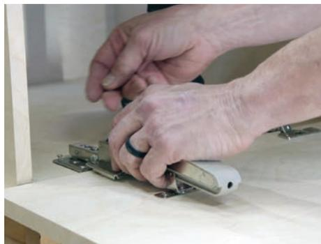
14) Mount the lid stay to the lid stay plate by tightening the rear screws and reinstalling the forward two screws.
