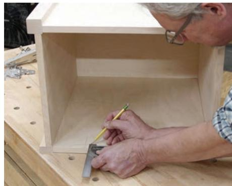
5) Draw a wide cross mark on the hinge centerlines on the cabinet body. These will locate the hinge plates.
